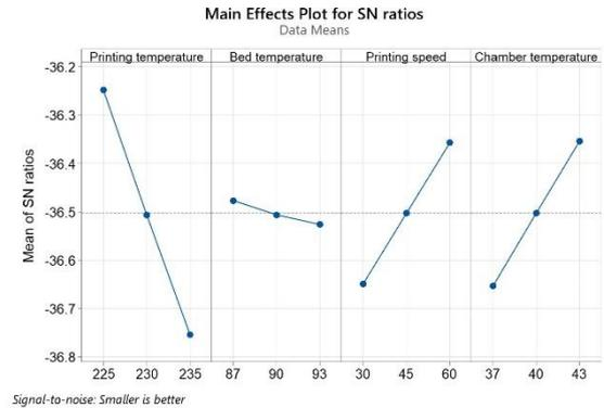
Figure 3. S/N ratio plot for residual stress
